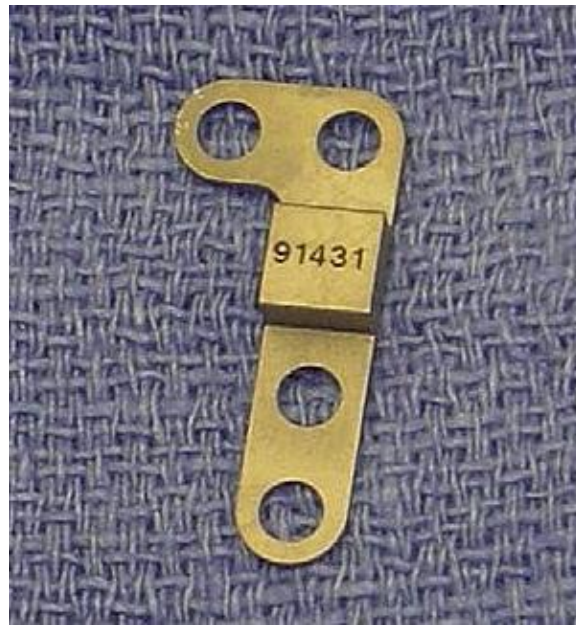
Figure 13: Arthrex OBW plate. It has many desirable features; a low profile design, a solid wedge that is offset from the wall of the plate. The wedge allows seating of the plate into a reproducible location and holds the osteotomy at a predictable gap distance. (31)
