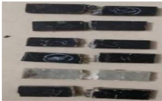
Fig. 4. Specimens after impact test
