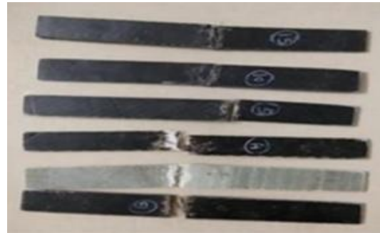
Fig. 3. Specimens after flexural test
